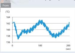
When a temperature sensor for a packaging machines is used, there is sometimes periodic temperature variation generated when there is a marked effect from the heat on the packaging materials side.
