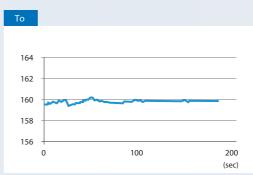
When the automatic filter adjustment function of the E5  $\Box$  D is used, this periodic temperature variation is suppressed automatically. It becomes possible to perform stable temperature control.
