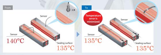
On a conventional machine, the temperature sensor was a little distance away from the sealing surface, so a difference occurred between the temperature of the sealing surface and the temperature that was actually being controlled. The temperature difference and failure rates increased in proportion to the packaging speed.
